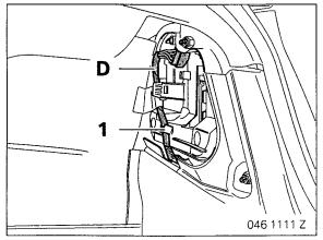
Clip the adapter cable **D** into the guide (1).
